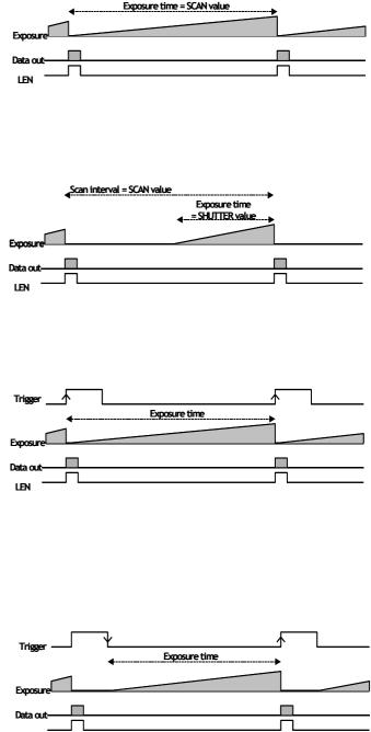
Fig. 11. Internal and external trigger modes.
